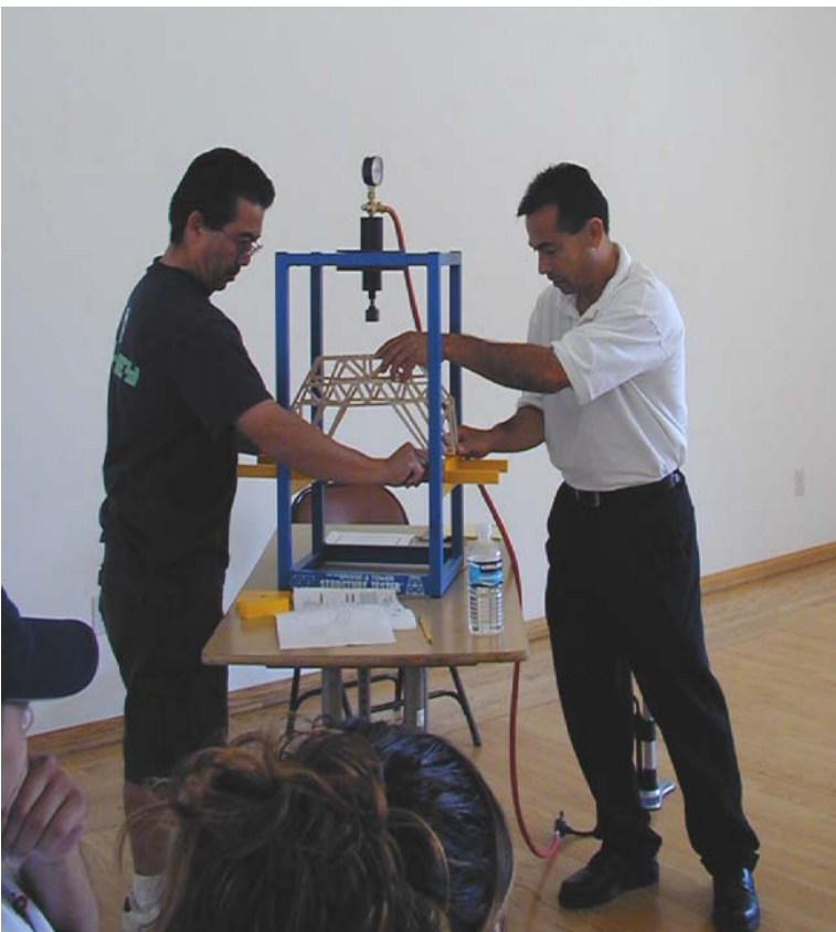
Instructors test the strength to weight ratio of a student's bridge.
